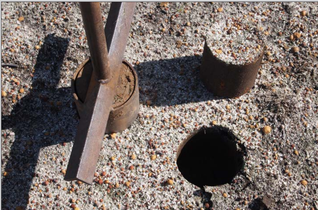
Figure 5.8 A metal soil corer with cross-bar for stepping on, and showing extracted core
