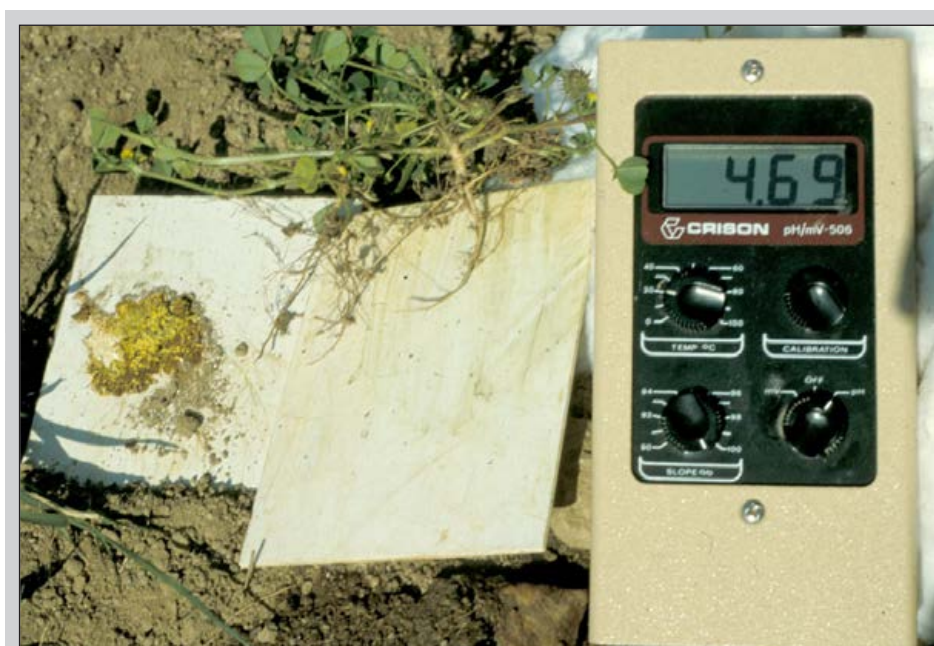
Figure 2.7 Soil pH is a valuable parameter to record. Note the yellow colour produced by the Universal Indicator pH kit which approximates to a soil pH of 4.69 as registered on the portable electronic pH meter after dilution of soil in 0.01 M CaCl 2 . This represents the lower limit for nodulation of annual species of Medicago , shown here collected in a natural environment on the Cyclades island of Tinos in Greece.
