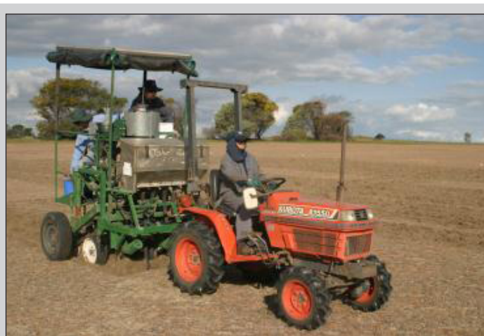
Figure 8.12 A precision seeding machine for sowing larger plots, such as for grain legume experiments.
